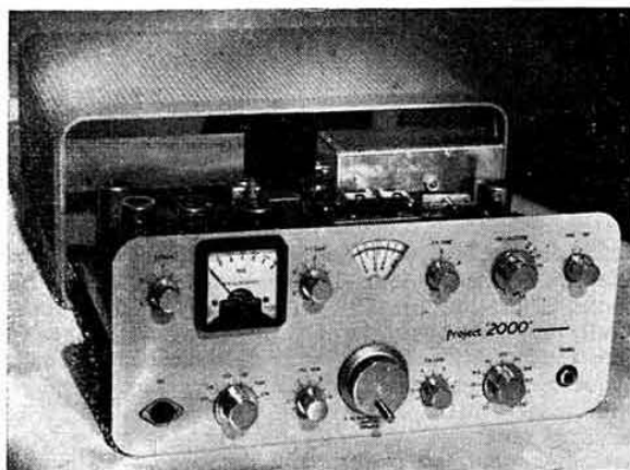
The first British s.s.b. transceiver is the K.W. Project 2000 manufactured by K. W. Electronics Ltd. of Dartford, Kent. The transceiver covers all bands from 10 to 160m in 200 kc/s sections. The p.e.p. input is 90 watts except on Top Band.
