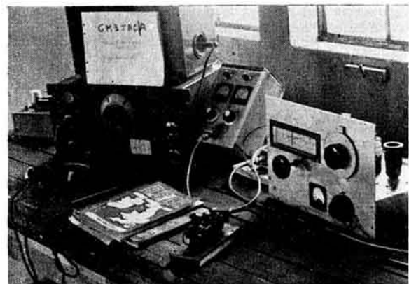
The equipment used at GM3UUU/P in Kincardine. To the right of the HRO is the aerial tuning unit and the EF91, EF91, TT11 transmitter.
